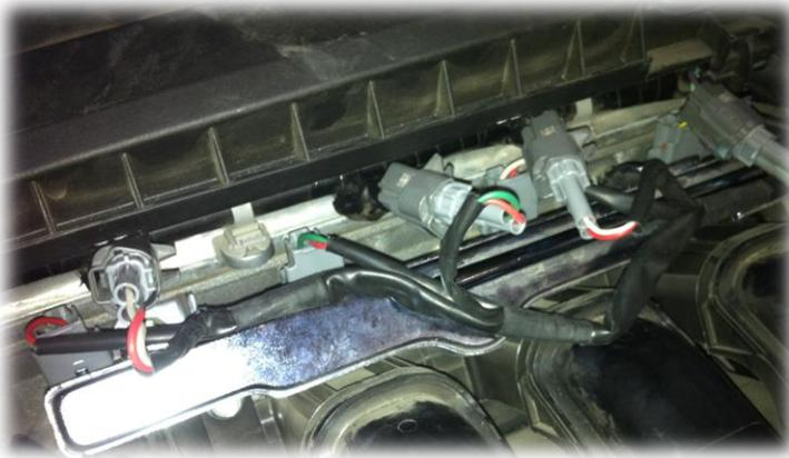
In a 6 cylinder engine with 2 harnesses, make sure that in the 1<sup>st</sup> harness the shortest connector will be connected to injector 1 and in the 2<sup>nd</sup> harness the shortest connector will be connected to the injector opposite of 1.
